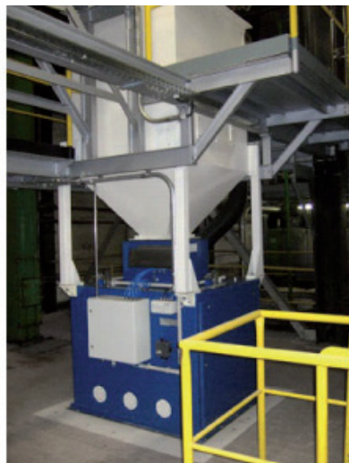
Electronic bulk scale model 34.144 acc. to ATEX directive. Site of operation: Riesaer Ölwerke Protection type:
